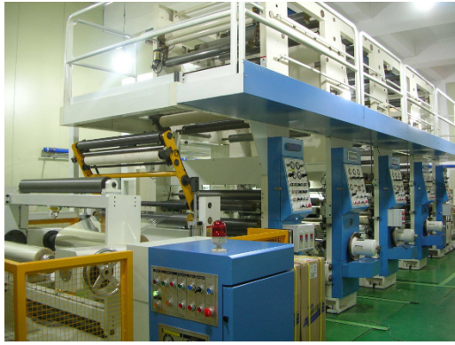
Fig. 1. Typical roll-to-roll gravure printing system.
